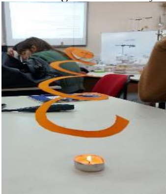
Figure 10 Visualizing air currents of heated air
