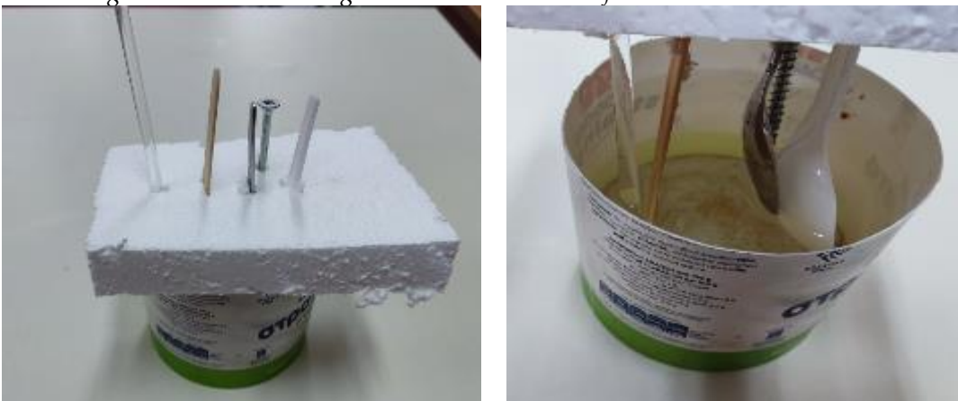
Figure 9 Examining which materials are good or bad conductors of heat
