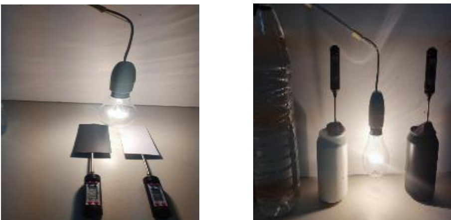
Figure 11 Examining heat transfer through radiation and measuring the temperature of dark-colored and light-colored bodies
